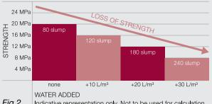
Fig 2 Indicative representation only. Not to be used for calculation.
