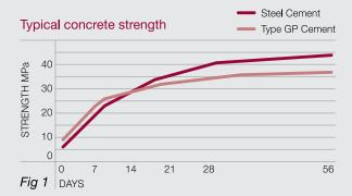
Standard laboratory mix and curing Water / cement ratio = 0.63, Slump = 80 Cement content = 300kh/m³, No admixtures used
