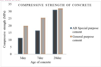
Figure 1: Compressive strength development of concrete. These concrete results are based on slump=80±10mm, cementitious
