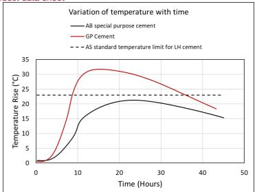
Figure 1: Variation of temperature with time in AB special purpose and GP cement
